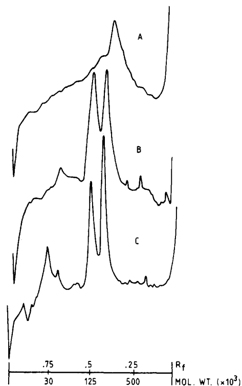
Figure 4. Electrophoretic mobility of sunflower protein without NaDodSO 4 : (A) alkali isolate; (B) water isolate; (C) salt isolate.
